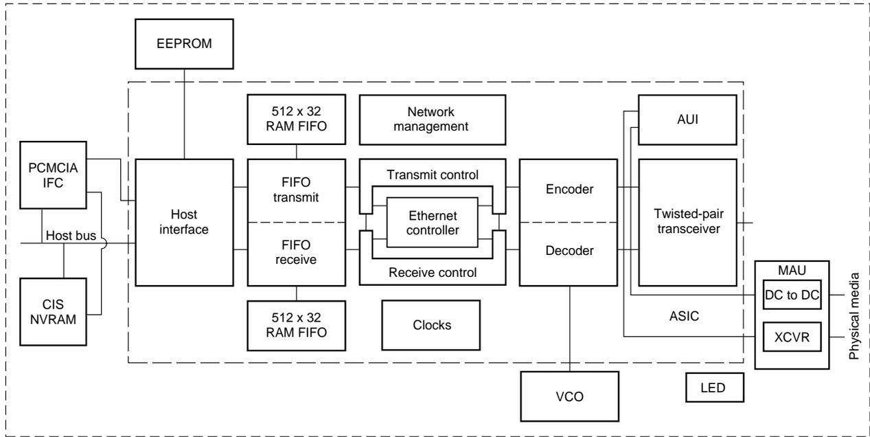
Figure 2-3. Block Diagram for PCMCIA (3C589)
