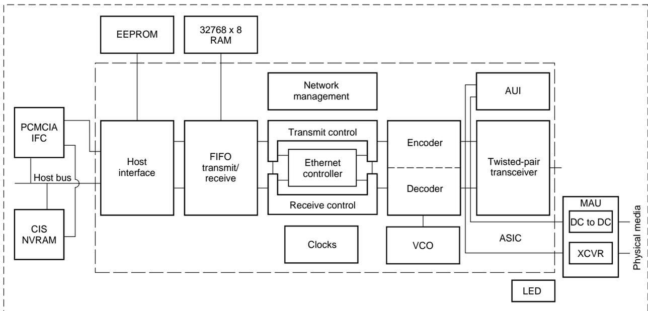
Figure 2-4. Block Diagram for PCMCIA (3C589B)
