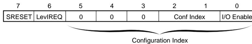
Figure 7-3. Configuration Option Register (3C589B)
