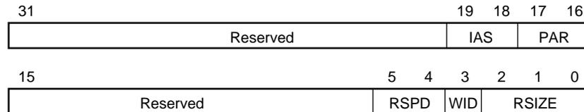
**Figure 7-27. Internal Configuration Register**
