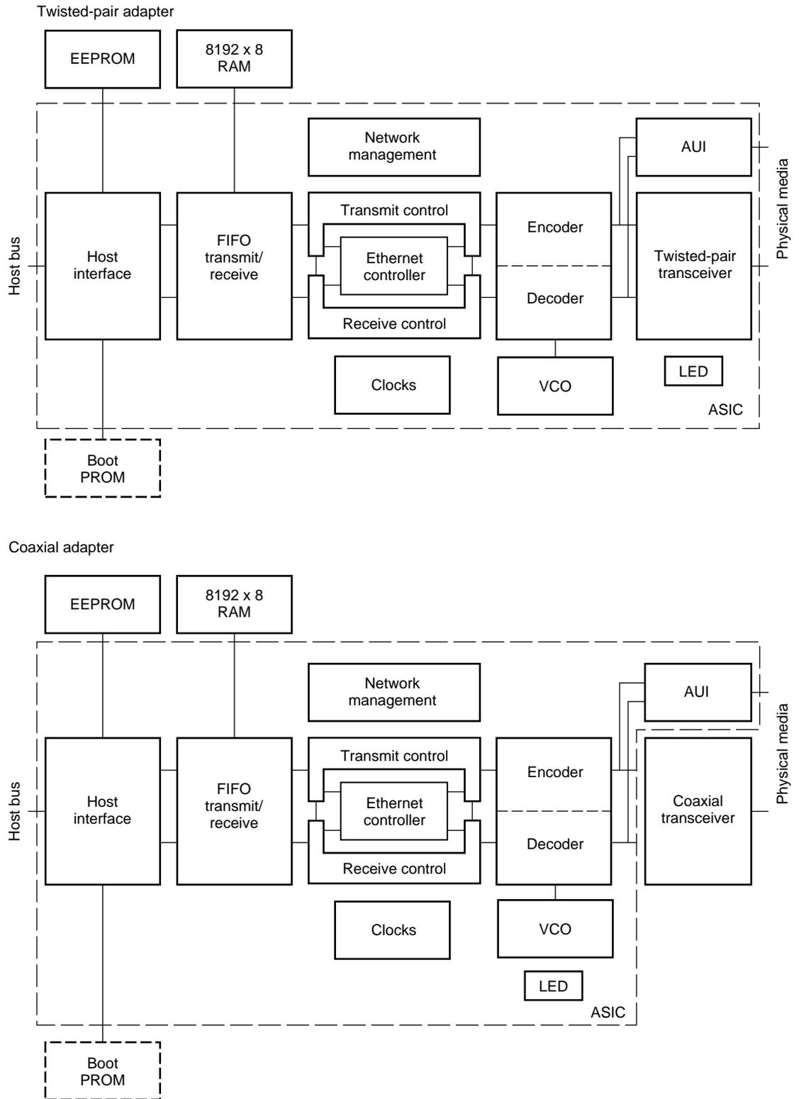
Figure 2-2. Block Diagrams for ISA (3C509B)
