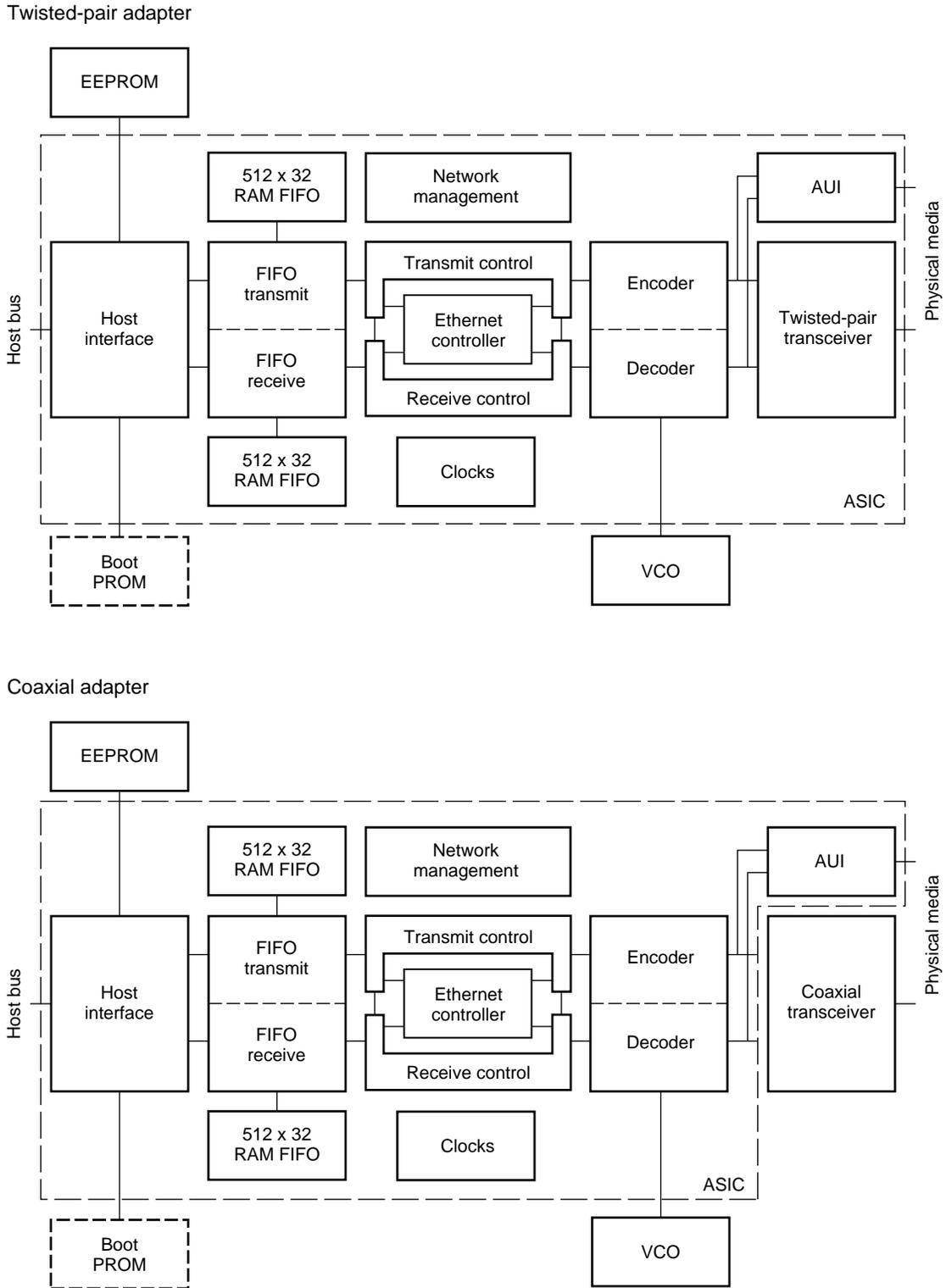
Figure 2-1. Block Diagrams for ISA, MCA, EISA (3C509, 3C529, 3C579)
